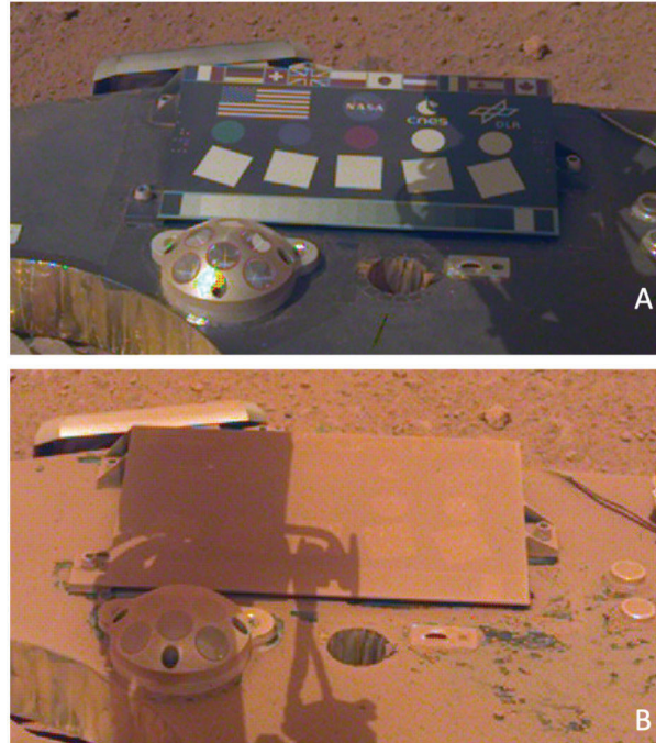
Fig. 19 IDC images of the calibration target on sol 12 (A) and sol 1238 (B) showing the accumulation of dust over the mission that almost completely obscured it
