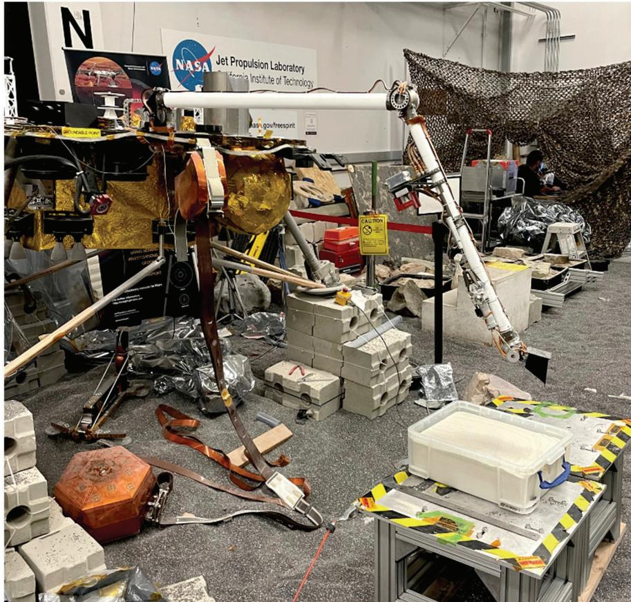
**Fig. 27** Picture of the engineering model lander, robotic arm, and scoop in the JPL testbed. Note the container of simulant below the arm as well as the SEIS and HP<sup>3</sup> models on the surface to the left. The IDC is on the forearm of the IDA and the ICC is mounted beneath the deck to the left (with red around the lens). Note the lander feet were placed on cinder blocks to enable end to end testing of arm activities that assisted the HP<sup>3</sup> mole and interacted with the surface
