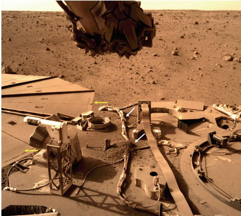
**Fig. 25** IDC image acquired on sol 1143 after the sixth solar array cleaning experiment showing the accumulation of soil on the western spacecraft deck (white arrows) from the first six soil dumps and the darkening of the western solar array (yellow arrows) from the dispersion of soil during the dumps
