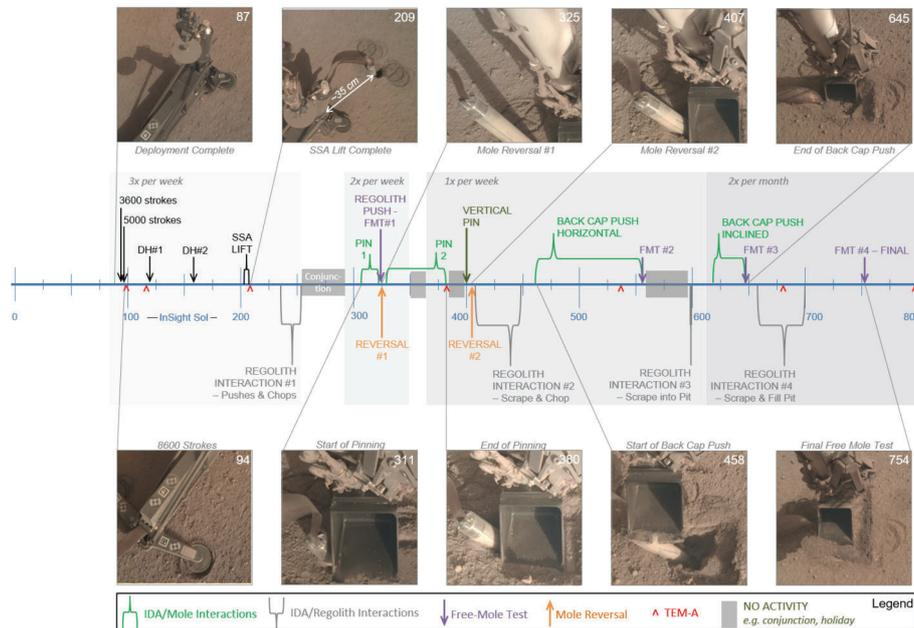
**Fig. 8** This linear timeline shows key periods (braces) and events (arrows and caret) of the mole recovery activity using the IDA from the end of SSA deployment (sol 87) to the final free-mole test (sol 764). Callout figures with sol numbers in the upper right show selected full-frame views from the IDC. Shaded background regions indicate changes in operational cadence
