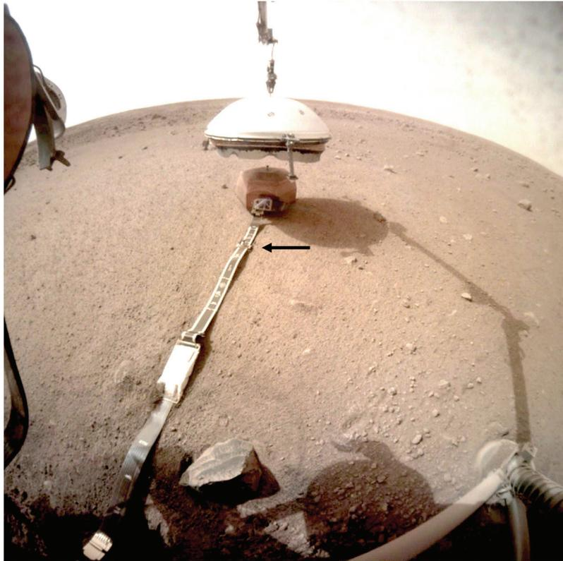
**Fig. 6** ICC image showing the WTS being lowered over SEIS on sol 66. Note location of the pinning mass (arrow), which is the ball on a post on the tether near SEIS that was later adjusted by the scoop on the IDA
