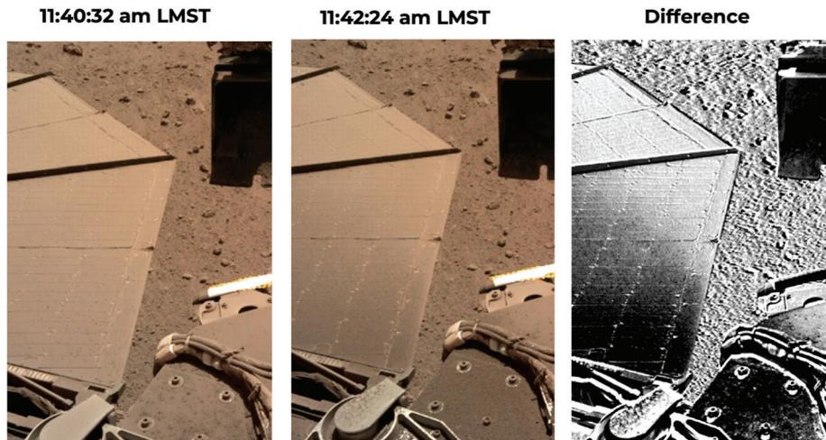
**Fig. 21** IDC images before (left) and after (middle) the main avalanche from the dump of soil on the northwestern edge of the lander on sol 884. Right image is the IDC differenced image showing areas where the surface has been darkened from soil that was dumped on the lander deck (right) and where dust has been removed from the west solar panel (left). For scale, the full diameter of the circular solar panels is 2.2 m
