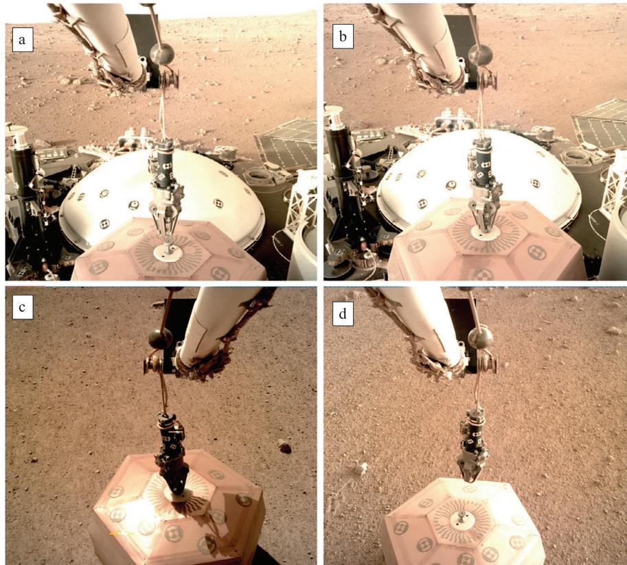
**Fig. 5** IDC images showing the four steps of deployment of SEIS. a) Aligning the IDA grapple over the grapple hook of SEIS on the deck. b) Grapple closed around the SEIS grapple hook. c) The instrument moved to the surface. d) The grapple unhooked from SEIS and moved above by the IDA. Note fiducial marks on the WTS (white dome) in a) and b) and on SEIS used to localize them after deployment
