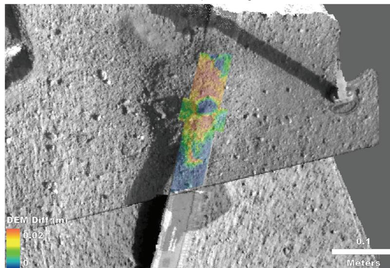
**Fig. 14** IDC differenced DEM (sol 877 minus sol 788) showing soil deposited on the SEIS tether after six dumps. Note circular blue spot in the middle of the tether length is an artifact over the pinning mass. Smoothing out that artifact indicates that 93% of the measured area of the tether is covered by 1 cm, 69% is covered by 1.5 cm, 50% is covered by 1.75 cm, and 30% of the tether is covered by 2 cm of soil
