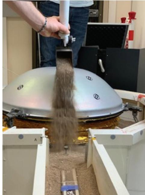
scoop onto the tether. There were two techniques for dumping soil on the tether. The first poured soil directly on the tether. The second poured the soil on the dome of the WTS so it slid off onto the tether close to the WTS. Dumping soil on the WTS was carried out to reduce the chance of soil pushing against the WTS skirt and potentially breaking its seal with the ground.
