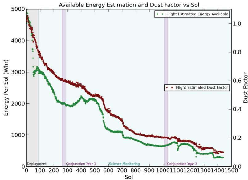
**Fig. 16** Plot of energy generated per sol (green) and the dust factor (red) versus time (sol) of the InSight lander. Power decreased exponentially and the dust factor worsened by  $\sim 90\%$  in the roughly 2 Mars years of the mission (1442 sols). Increased rates of change in dust factor (and power production) correlate with periods of higher atmospheric opacity associated with dust storms
