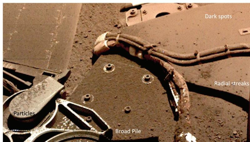
**Fig. 22** Close up of the dump site on the northwestern part of the lander deck and the edge of the western solar panel on sol 884. Note some individual granules (of order mm) can be resolved as well as larger clods. Note radial streaks in circular impact site between the cables
