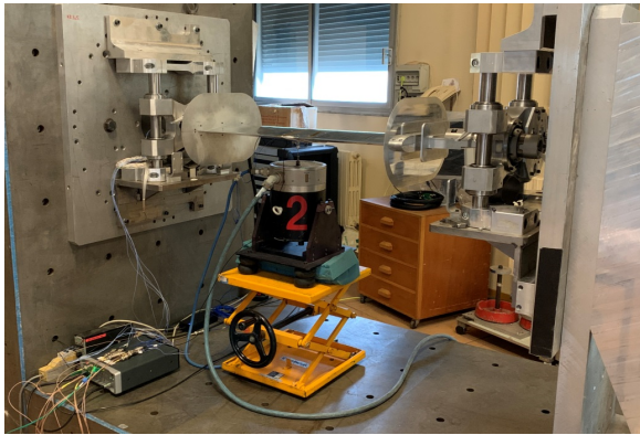
Figure 3: Experimental setup for the preliminary laboratory testing of the structural modes of the model.
