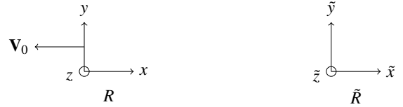
Figure 3: Moving frame R at a velocity \mathbf{V}_0 with respect to the fixed frame \tilde{R} .
