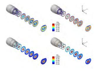
Figure 4: Viscous and thermal anergy generation at successive stations downstream of the engine (ADP/BF) for the medium (left) and fine (right) grids.
