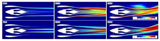
Figure 10: Viscous anergy (top) and thermal anergy (bottom) fields at different operating points (BF / Medium grid).
