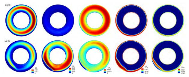
Figure 8: Exergy fluxes and anergy generation downstream of the OGV for the low-speed operating point at two different angles of attack (BF / Medium grid).
