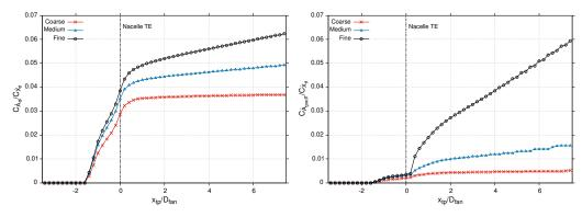
Figure 5: Evolution of viscous and thermal anergy by the variation of the c.v. downstream limit (ADP/BF).
