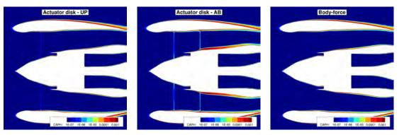
Figure 6: Viscous anergy close to the engine axis for the AD-UP, AD-AB and BF computations (ADP / Medium grid).
