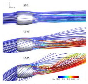
Figure 11: Streamribbons coloured by viscous anergy generation for the three different operating points of the ASPIRE engine (BF / Medium grid).
