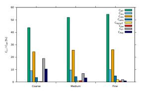
Figure 3: Grid convergence of the exergy balance using a body-force model of the fan-OGV at the ADP operating point, for  $x_{tp}/D_{fan} = 1.0$ .
