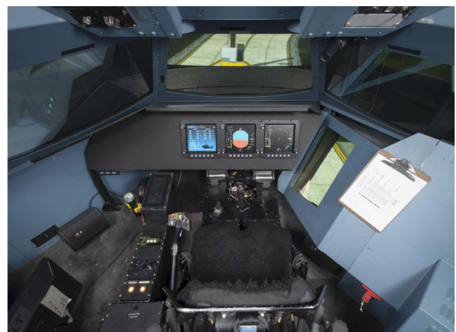
Figure 5. R Cab cockpit emulating a utility class UH-60 sized helicopter.
