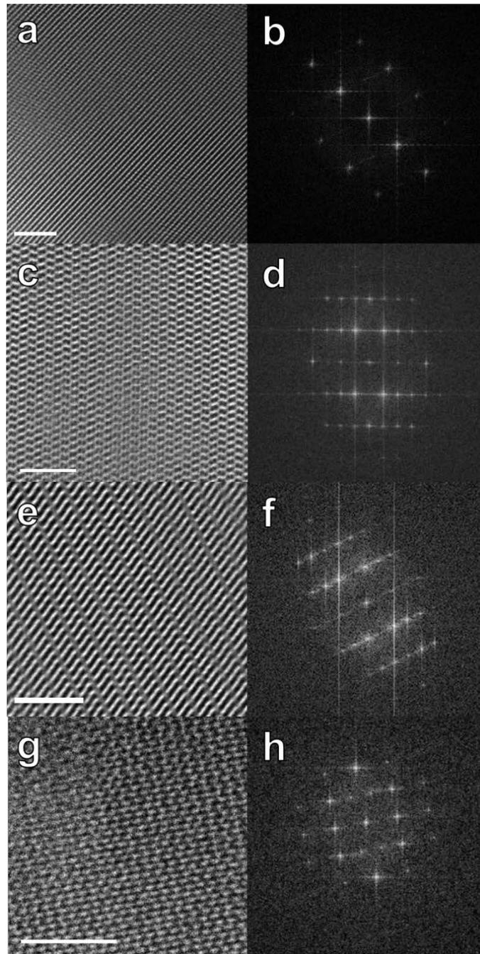
**Figure S8:** Direct space and Fast Fourier Transformed (FFT) images of superhelical protein origami crystals. In these particular areas, highly regular and periodical moiré patterns reveal the overlap of two or more crystals oriented each along different zone axis. The FFT shows the collection of spots equivalent to the overlapped electron diffraction patterns of all the zones axis.
