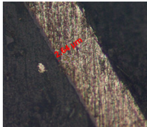
Figure 8. Microscopic section of the strip after seven cycles of 72 h at 440 °C.
