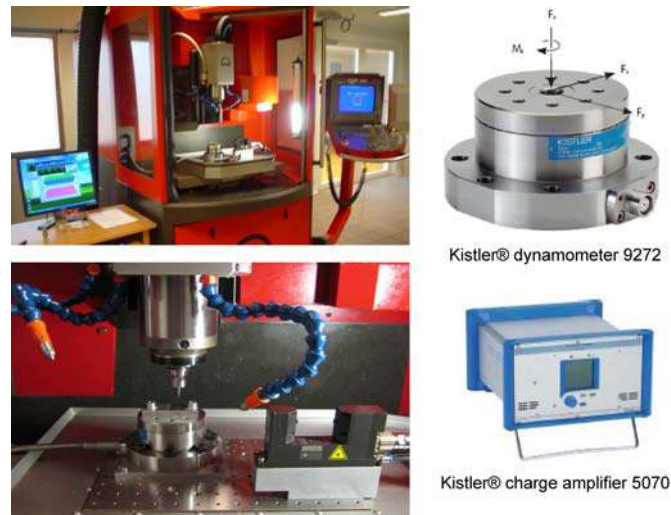
Fig.11. Experimental set up to measure the cutting forces in milling
