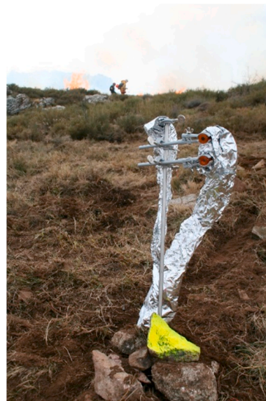
Fig. 3. Radiant and total heat flux sensors and thermocouple fixed on supporting rod and protected by aluminum foils.
