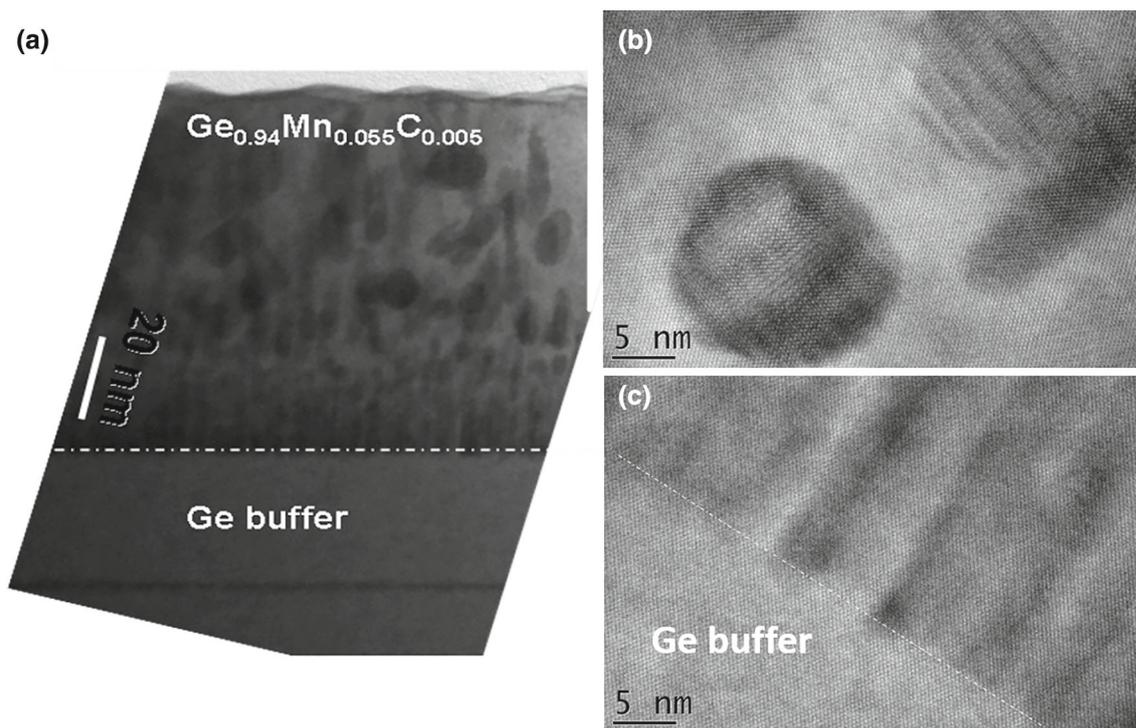
**Figure 2.** (a) Typical TEM image of  $\sim 80$ -nm thick  $\text{Ge}_{0.94}\text{Mn}_{0.055}\text{C}_{0.005}$ ; (b) high-resolution TEM micrographs of the  $\text{Ge}_{0.94}\text{Mn}_{0.055}\text{C}_{0.005}$  film and (c) the region around the interface between Ge buffer and  $\text{Ge}_{0.94}\text{Mn}_{0.06}$  film.
