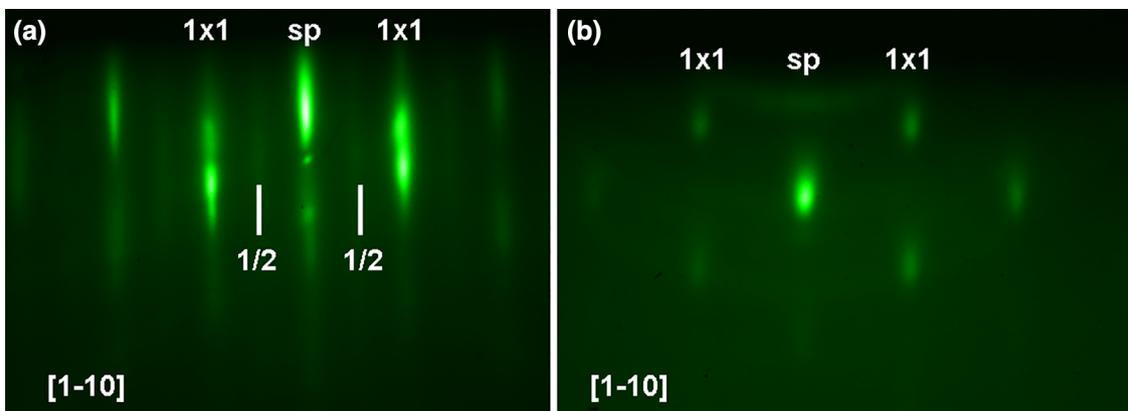
**Figure 1.** RHEED patterns taken along  $[1-10]$  azimuth (a) during the growth of carbon-free  $\text{Ge}_{0.94}\text{Mn}_{0.06}$  nanocolumns and (b) during the  $\text{Ge}_{0.94}\text{Mn}_{0.055}\text{C}_{0.005}$  growth.
