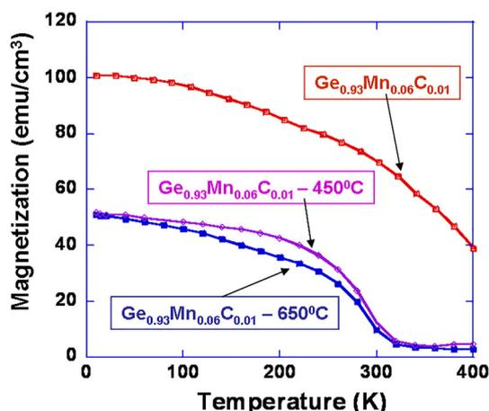
**Figure 5.** Evolution of magnetization vs. temperature of a  $\sim 80$ -nm thick  $\text{Ge}_{0.94}\text{Mn}_{0.05}\text{C}_{0.01}$  film after annealing at 450 and 650°C for 20 min. For comparison, magnetization of as-grown sample is shown.
