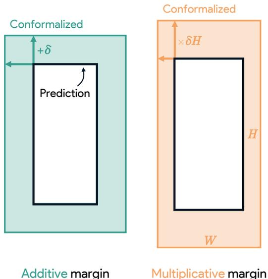
Figure 2: **Effect of margin systems used.** An additive margin is a number of pixels to add, while a multiplicative margin is a proportion of the width/height to add. The additive one may lead to comparatively a smaller effect on foreground boxes and larger on background (smaller traffic signals) boxes, and the opposite applies for multiplicative margins.
