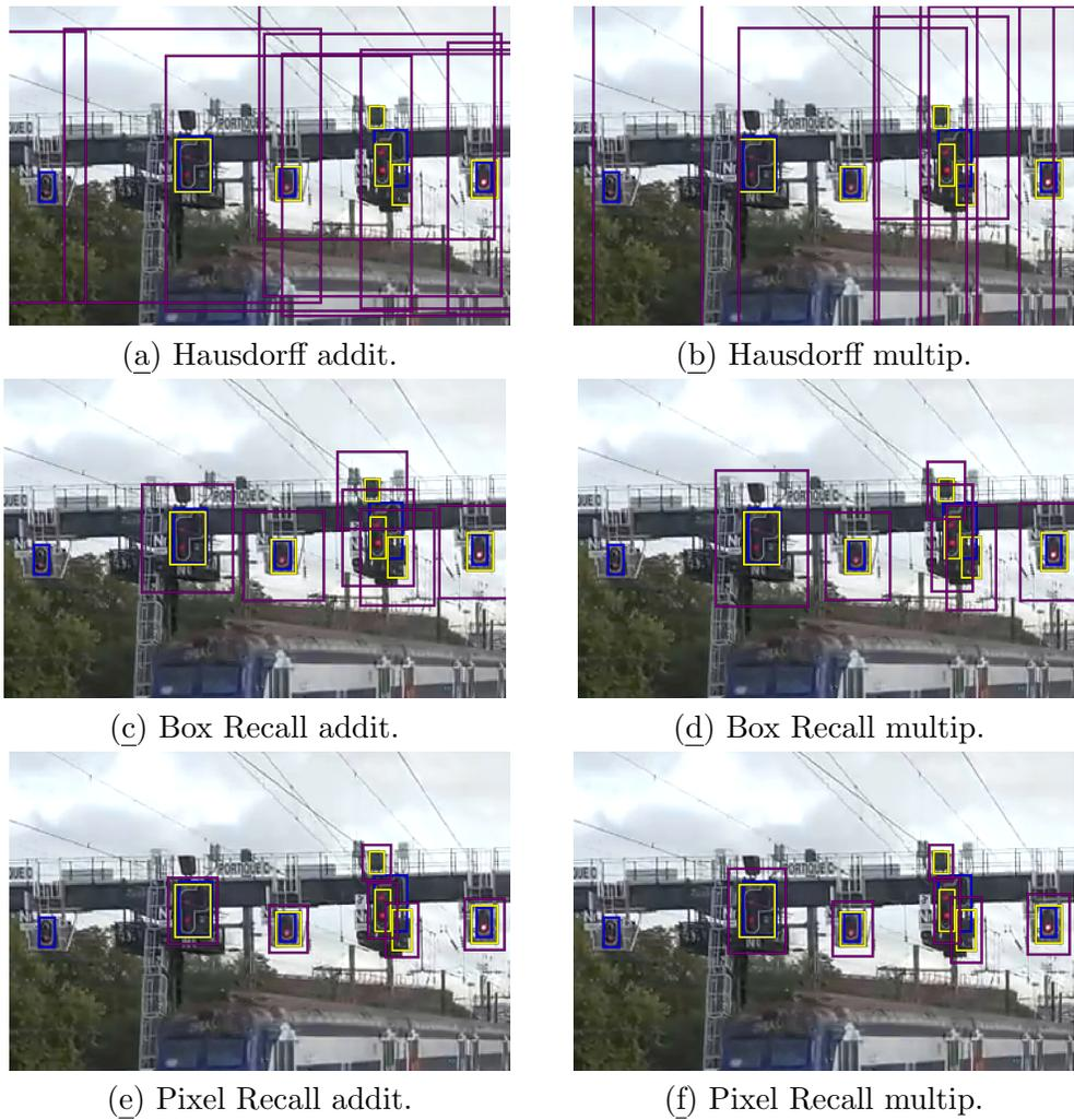
Figure 5: **Image-wise conformalization on an image with several traffic signals (including true and false positives, and false negatives.** Bounding boxes as predicted by the DiffusionDet predictor in yellow, conformalized boxes in purple and ground truth in blue. Cropped for readability.
