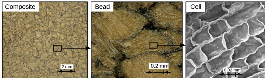
Figure 1: Agglomerated cork: a multi-scale cellular material.
