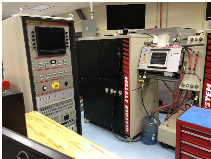
Figure 1. The Gleeble-3800 thermomechanical simulator system used for this study
