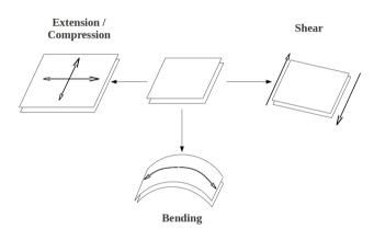
Figure 4. The microcapsule shell deformations: dilation, shear and bending resistances.
