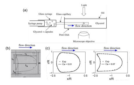
**Figure 9.** Microcapsules characterization in the confined flow. (a) Schematic of the experimental setup (from Ref. [88]). (b) The profile of a deformed microcapsule in the capillary flow (from Ref. [89]). L,  $L_a$ ,  $L_p$  and  $L_r$  are the geometric parameters which can be extracted from the image. R is the radius of the channel. (c) Comparison of the experimental (dotted line) and numerical (continuous line) profiles (from Ref. [63]).
