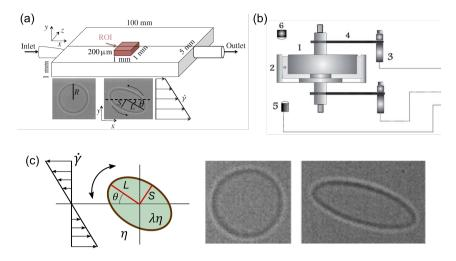
**Figure 10.** Microcapsule deformation in shear flow. (a) Approximately linear shear flow (ROI) in a high aspect ratio channel (from Ref. [43]). (b) Schematic of the Couette-like rheoscope. 1—inner cylinder, 2—outer cylinder, 3—motor drive unit, 4—belts, 5—microscope objective, 6—light source. (from Ref. [42]). (c) The microcapsule aligned and deformed in the shear flow. The viscosity ratio between the interior and exterior is  $\lambda$ . Images are from Ref. [43].
