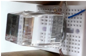
Figure 3. A prototype LYSO crystal readout by a Silicon photomultiplier. The tapered design was selected to cover a larger solid angle, and increase photopeak efficiency compared to a parallelepiped. The crystal is 3 cm along the long axis. This picture does not feature any crystal wrapping.
