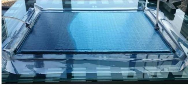
**Figure 2:** Vacuum bag resin transfer moulding of flax reinforcement using Infugreen 810
