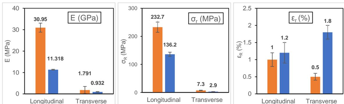
Figure 3. Longitudinal and transverse hygro-elastic mechanical properties at break of dry and wet unidirectional biocomposites: Tensile Modulus  $E$ , Stress at break ( $\sigma_r$ ) and strain at break ( $\varepsilon_r$ ) (orange for dry state and blue for wet state)
