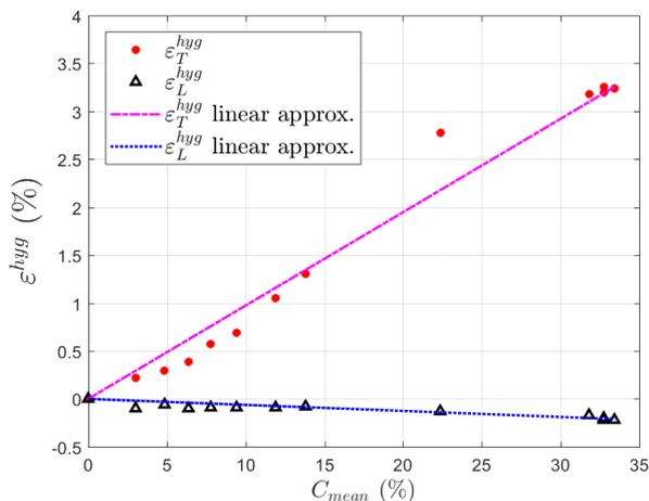
Figure 2: Evolution of longitudinal and transverse hygroscopic strains. Red and black dots represent experimental data and continuous lines represent theoretical results from model.
