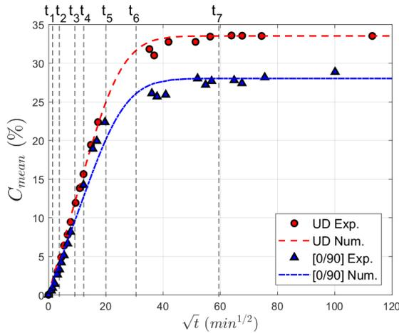
Figure 6: Evolution of the experimental and modelled mean moisture content for both ply sequences. Error bars on the experimental results are not represented for the sake of clarity but can be found in Fig. 1.
