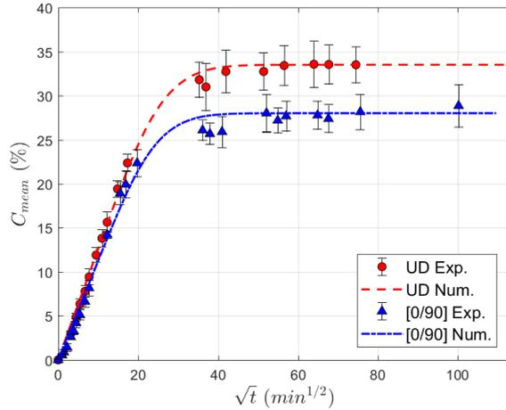
Figure. 1. Diffusion kinetics of unidirectional  $[0_6]$  and asymmetrical  $[0_1, 90_5]$  biocomposite laminates. The dashed curves represent the evolution of numerical mean moisture content  $C_{mean}$  given by the Fick model
