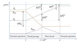
FIGURE 1. Idealized response of autonomous power systems to a cloud-passage event.
