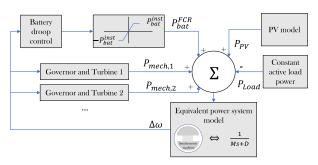
FIGURE 4. Power system model implemented in OpenModelica.
