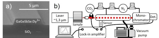
Fig. 2. a) Scanning electron microscope picture of a Dy<sup>3+</sup>-doped GaGeSbSe ridge waveguide. b) Optical set-up enabling CO<sub>2</sub> concentration-dependent PL measurements,
