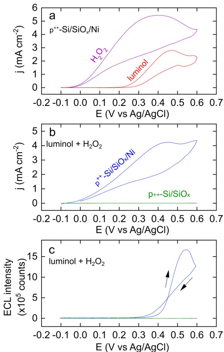
**Figure 3.** a) CVs recorded in the dark on  $p^{++}$ -Si/SiO<sub>x</sub>/Ni in a pH 13 aqueous solution containing 33 mM H<sub>2</sub>O<sub>2</sub> (purple curve) or 10 mM luminol (red curve). b) CVs recorded in the dark in both 33 mM H<sub>2</sub>O<sub>2</sub> and 10 mM luminol (pH = 13) on  $p^{++}$ -Si/SiO<sub>x</sub>/Ni (blue curve) and  $p^{++}$ -Si/SiO<sub>x</sub> (green curve). c) Corresponding ECL intensity/potential profiles. Scan rate: 50 mV s<sup>-1</sup>.
