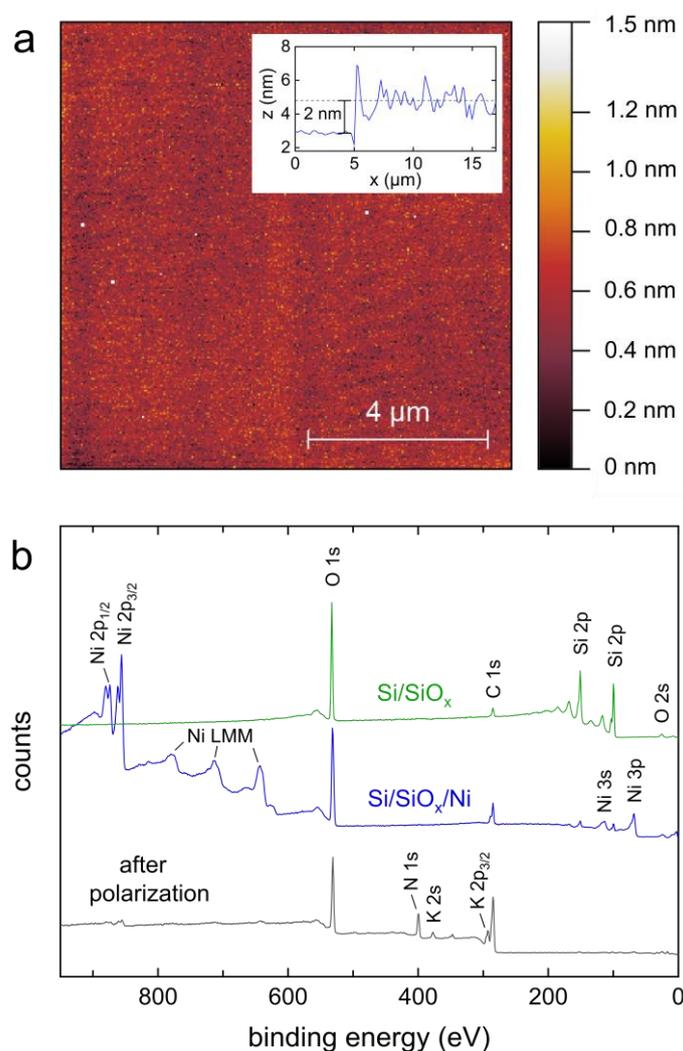
**Figure 2.** a) AFM picture of  $p^{++}$ -Si/SiO<sub>x</sub>/Ni. Inset: AFM height profile of the Ni thin film onto  $p^{++}$ -Si/SiO<sub>x</sub> after a lift-off process. b) XPS survey spectra of  $p^{++}$ -Si/SiO<sub>x</sub> (green),  $p^{++}$ -Si/SiO<sub>x</sub>/Ni (blue), and  $n$ -Si/SiO<sub>x</sub>/Ni (black) after potentiostatic polarization at 0.2 V for 4.5 h under IR illumination in the ECL electrolyte.
