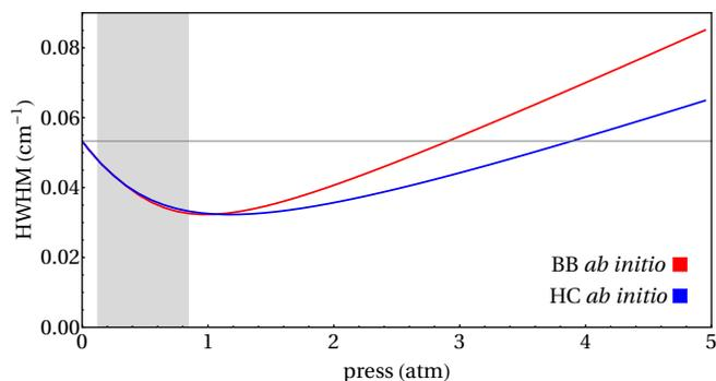
FIG. 5. Pressure dependence of the half width at half maximum (HWHM) of a spectral line. We consider two velocity-changing collision models: the *ab initio* billiard-ball model (BB *ab initio*) and the *ab initio* hard-collision model (HC *ab initio*). The gray zone marks the partial pressure range of Ar covered in our experiments. It is seen that in the range considered by us, the HWHM of the two line-shape models is almost the same.
