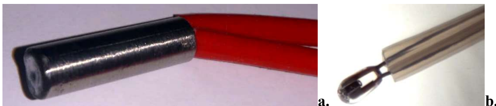
Fig. 3. Cartridge heater for filament melting (a) and thermistor for temperature measurement (b).
