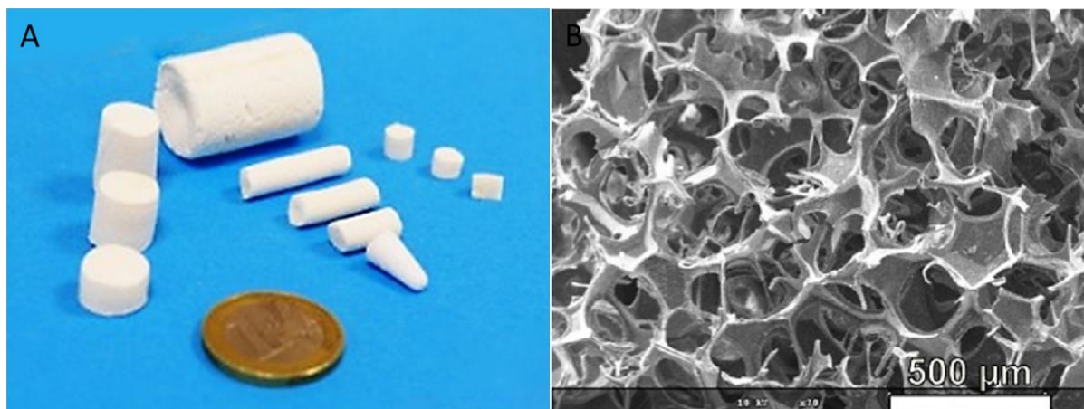
Figure 4. Gelatin/BAG hybrid scaffolds, a) under different shapes; b) observed in scanning electron microscopy. [164]
