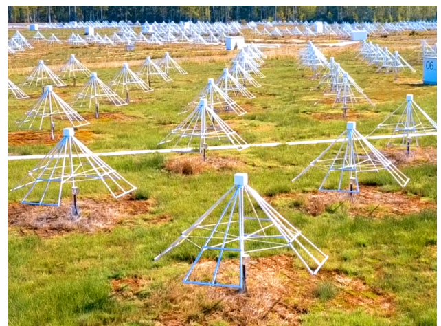
Figure 1. NenuFAR antenna field in Nançay. Each LWA-like antenna is mounted above a 3\text{m} \times 3\text{m} metal grid (ground plane). The custom-made preamplifier is in the white box at the top of each antenna.
