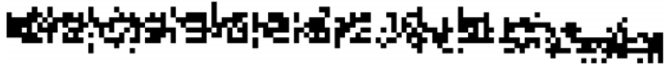
Fig. 6. Physical bitmap representation of the memory under test. In this figure, a SEL is propagated to a well-tap defined region of the memory. Pixels in white denote noncorrupted bit-cells, while pixels in black correspond to corrupted cells.
