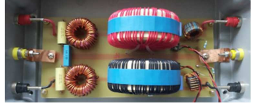
Fig. 4. The experimental DC LISN.
