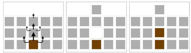
Fig. 8. From left to right: rust presses against the voxels above and around it; When the above voxels reach a threshold, they are displaced; A new rust voxel is instantiated at the vacant position.
