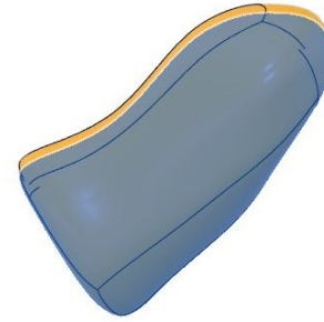
Fig. 7 Superposition of the volume of the thumb in the desired open opposite position (in yellow) and the volume obtained by rotation of the thumb in the opposite closed position (in grey)
