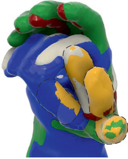
Fig. 6 Superposition of the four scanned surfaces and placement of a volume (in yellow) in correspondence of the surfaces
