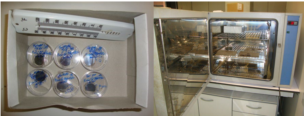
Figure 7. The six alloys immersed in six separated cells (left) and their introduction in the oven for the one month stay at 37°C (right).
