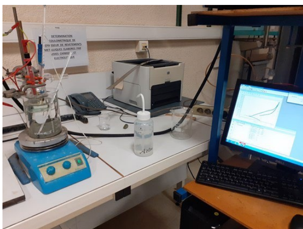
Figure 8. The {three electrodes} cell (left) conceived as a water bath (electrolyte and electrodes immersed), and a potentiostat driven by a software hosted in a computer (right).
