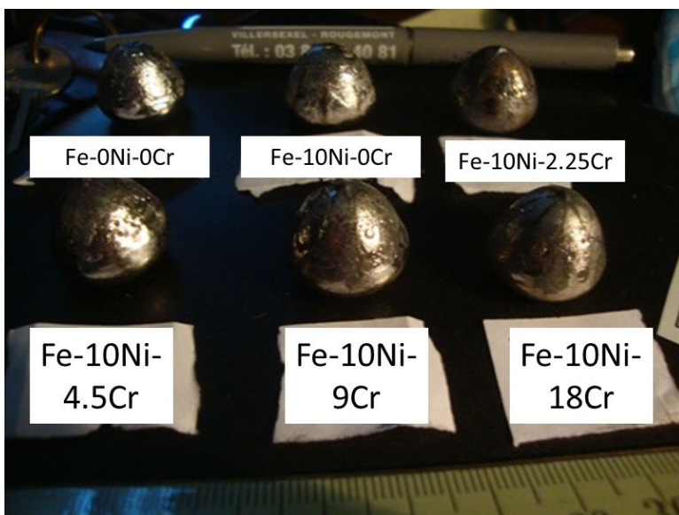
Figure 3. The six ternary alloys produced as 20g–weighing ingots.
