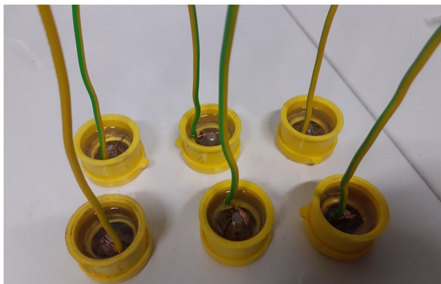
Figure 5. The second parts of the ingots prepared as working electrodes.
