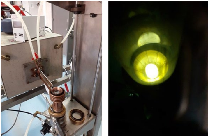
Figure 2. After having placed the Fe, Ni and Cr metallic parts in the copper crucible (left), induction heating in a pure Ar atmosphere induced the melting of the mix (right).
