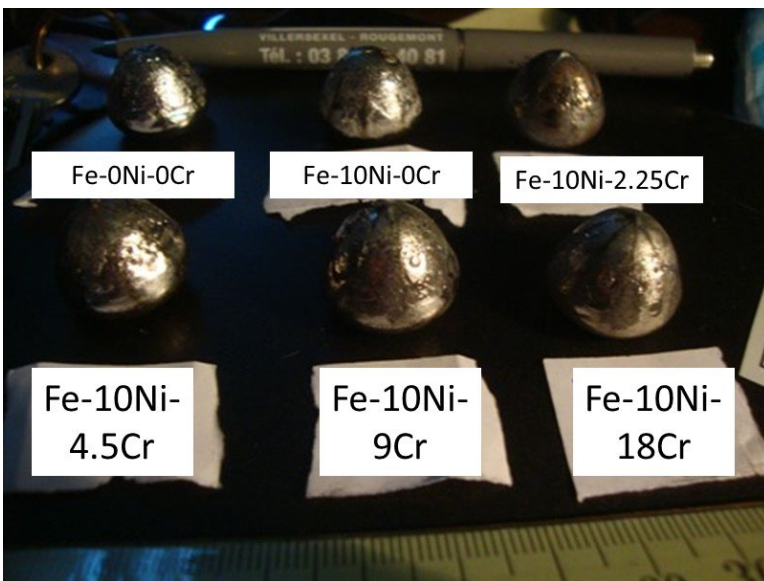
Figure 3. The six ternary alloys produced as 20g–weighing ingots.
