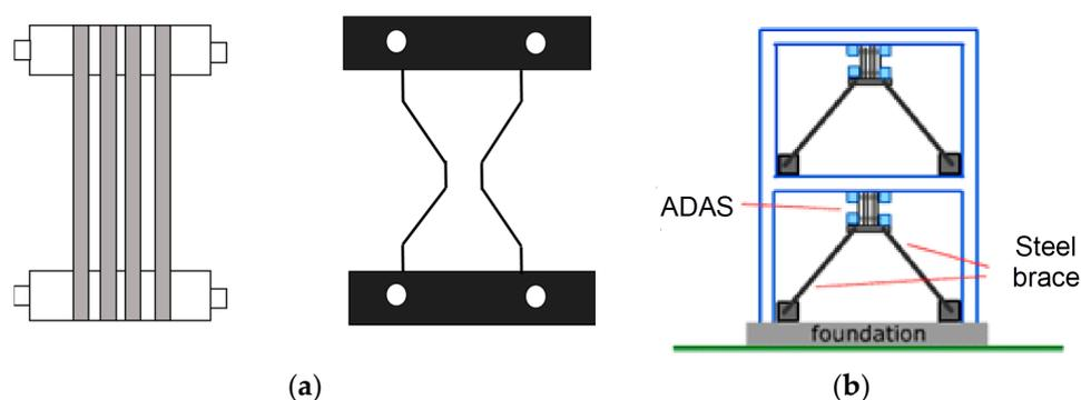
**Figure 9.** (a) Description of ADAS damper, (b) two story frame with ADAS damper.
