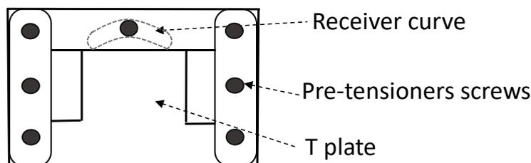
**Figure 5.** Construction of the improved Pall friction damper proposed by Wu et al.
