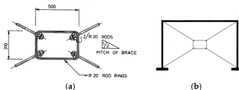
**Figure 8.** Premier metallic damper. (a) description of the rectangular metallic damper, (b) one story frame with the metallic damper.
