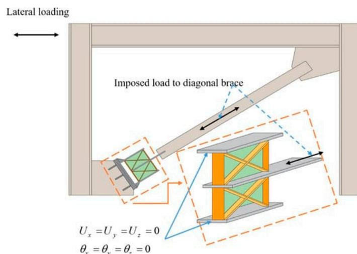
Figure 10. A new MD that improves the behavior of the shear dampers [129].
