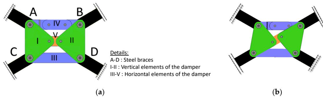
**Figure 6.** Construction of the improved Pall friction damper proposed by Papadopoulos, (a) inactive damper, (b) activation of the damper.
