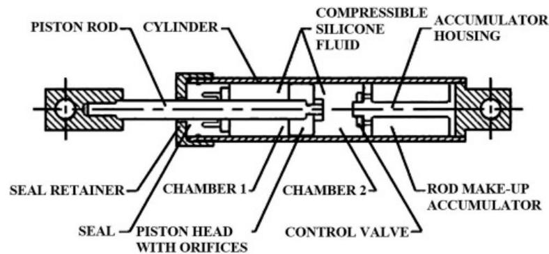
**Figure 13.** Longitudinal section of a typical Viscous fluid damper.
