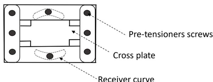
Figure 3. Pall friction damper.
