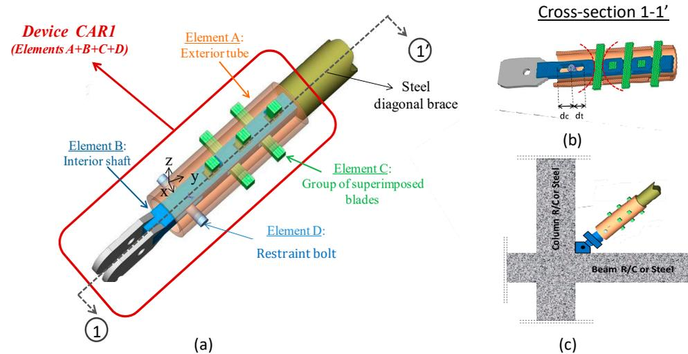
**Figure 7.** Description of CAR1 damper, proposed and investigated by Titirla et al. [73]. (a) The proposed steel device CAR1, (b) the cross section 1-1' of the device CAR1, (c) connection of device in RC or Steel structures.
