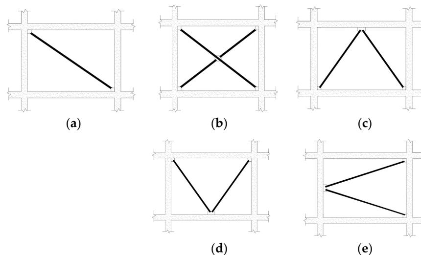
**Figure 1.** Centrally Braced Frames: (a) single diagonal bracing, (b) cross bracing, (c)  $\Lambda$  bracing (chevron), (d) V bracing (chevron), (e) K bracing.
