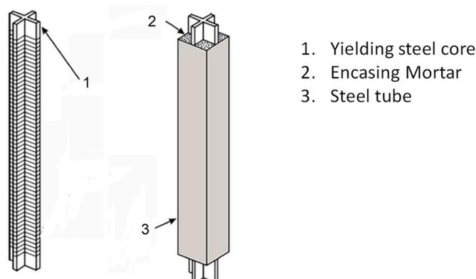
Figure 11. Construction of a buckling-restrained brace.
