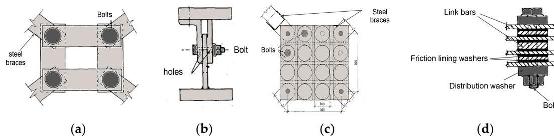
**Figure 4.** Improvement of PFD proposed by Anagnostides et al.: 1. three plates damper with high-strength bolts (a) longitudinal section, (b) cross-section. 2. twelve friction joints incorporating frictional washers (c) longitudinal section, (d) cross-section.
