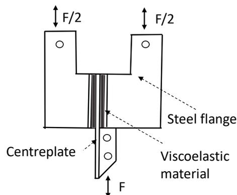
**Figure 15.** Improvement of Viscous Damper.
