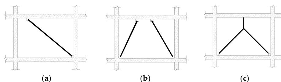
**Figure 2.** Several schematic models with eccentric bracing systems: (a) single diagonal bracing with eccentricity, (b) double diagonal bracing with eccentricity, (c)  $\Lambda$  bracing with eccentricity.
