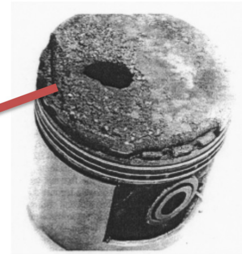
piston damaged by strong knock (LLNL)
