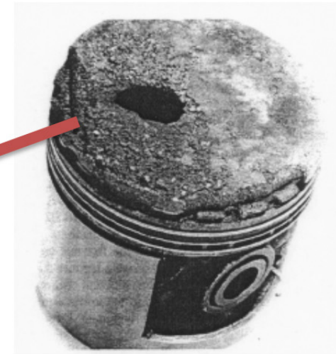
piston damaged by strong knock (LLNL)
