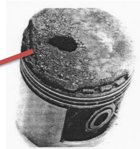
piston damaged by strong knock (LLNL)
