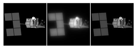
Fig 12 Left and center: True object and image for simulated satellite observation,  $256 \times 256$  cropped from  $512 \times 512$  (Figure 8). Right: restored object, also cropped.
