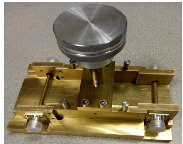
FIGURE 5. Test cell design is not connected to the VNA without the SUT.
