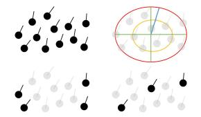
**Fig. 3** The display types of the swarm (from [32]): in the top left, the *full information* display, *i.e.* each agent's direction; in the top right, the swarm's centroid (at the intersection of the green cross), along with a bounding ellipse (in red) and another ellipse (in yellow) representing the robot positions median; and in the bottom left and right, only some leaders' direction.
