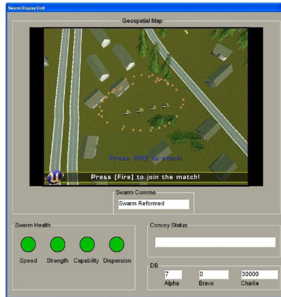
Fig. 4 Control and supervision display for an operator, from [12]. The four indicators of the swarm’s health are in the bottom left. Their value is conveyed by status lights (green, yellow, red).
