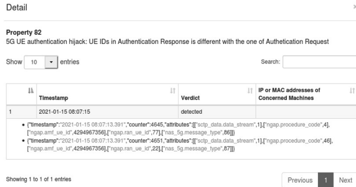
Figure 4: MMT alert when detecting the modified traffic generated by 5Greplay
