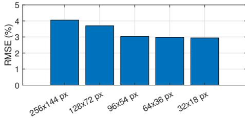
Figure 17: Impact of cell size on SmartPhOx v1 performance.
