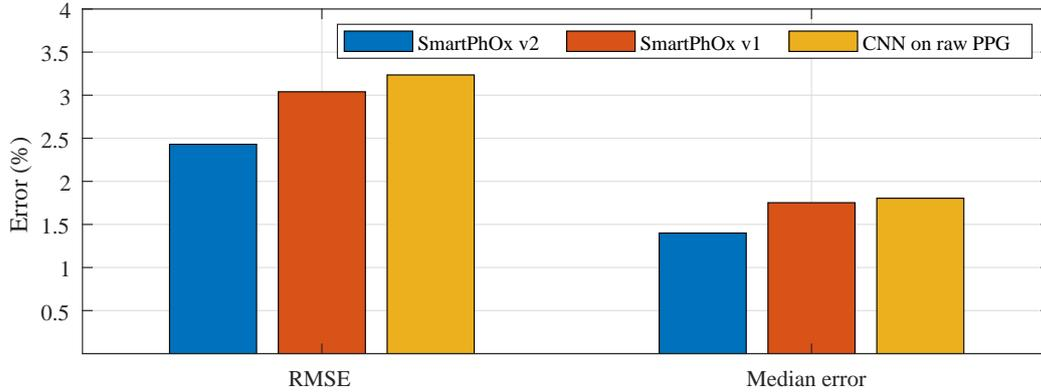
Figure 16: SmartPhOx v1 and SmartPhOx v2 vs the CNN proposed by [16]. Training the neural network on the RR map leads to better results when compared to training a CNN on the raw PPG signals.
