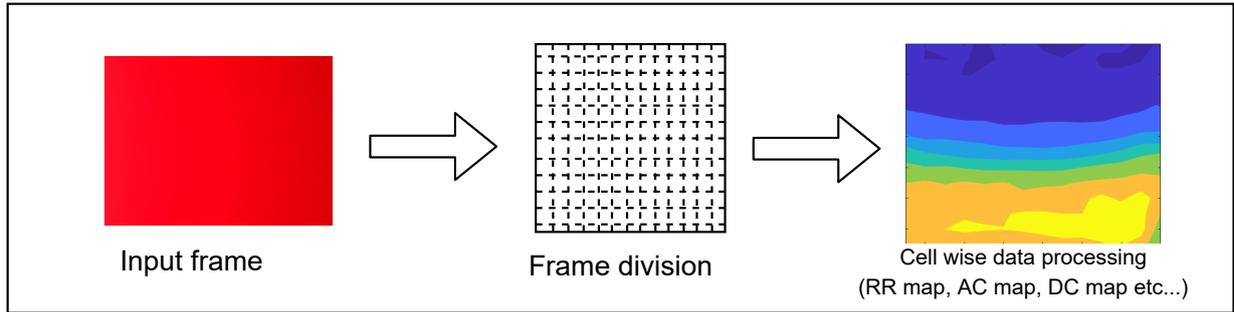
Figure 5: Virtual sensor array principle. From one single large frame to cell wise data processing, resulting in RR map, AC map, DC map etc.
