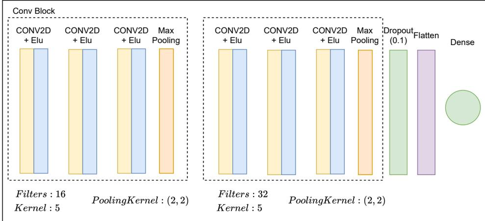
Figure 10: SmartPhOx v2 CNN architecture with best hyperparameters.
