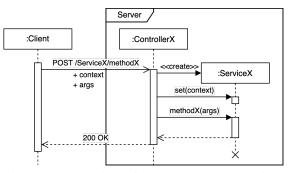
Figure 1: Wrapping of legacy RMI service into new Spring controller
