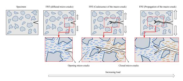
Figure 1: Concept of the crack evolution in the FPZ for heterogeneous media.
