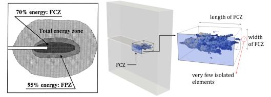
(a) Definition of FCZ and FPZ in experi- (b) Cuboid that envelops elements carrying a crack opening value larger ments than 0.001 mm
