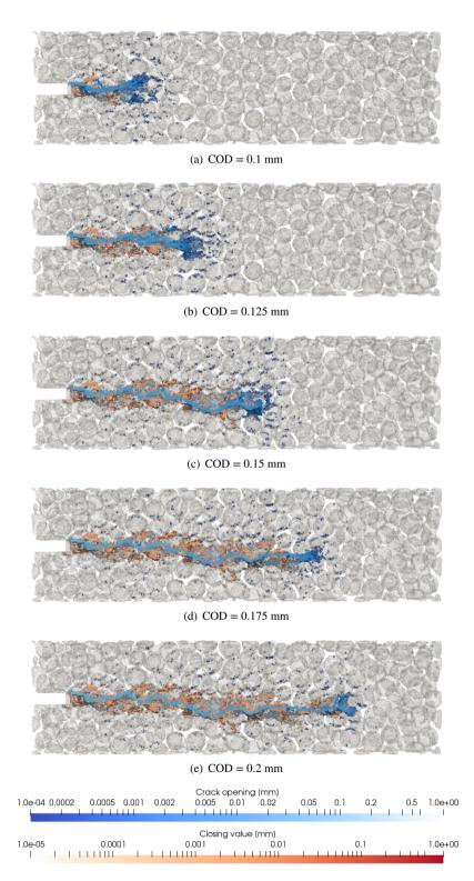
Figure 18: Crack pattern evolution of  $d_{max} = 10 \text{ mm r3}$  concrete: crack openings and crack closures.
