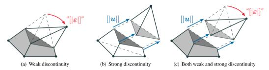
Figure 3: Three elements carrying different types of enhancements.
