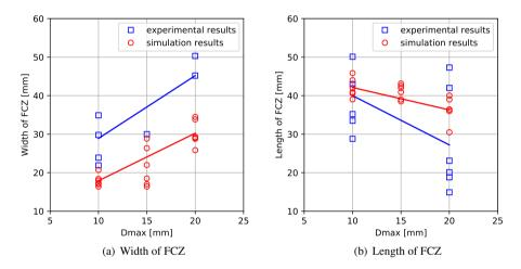
Figure 14: Relationship between d<sub>max</sub> and dimensions of FCZ at peak load in experiments and in numerical simulations.
