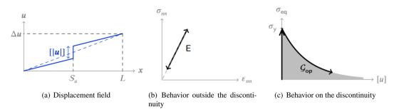
Figure 4: Behavior of the strongly enhanced element at the crack opening phase.
