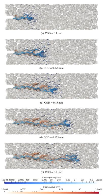
Figure 11: Front view of the crack pattern evolution of  $d_{max} = 10 \text{ mm r1}$  concrete: crack openings and crack closures (aggregates marked in transparent gray).
