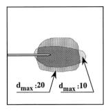
Figure 15: Relationship between  $d_{max}$  and dimensions of FCZ at peak load in numerical simulations.
