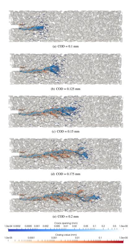
Figure 17: Crack pattern evolution of  $d_{max} = 10 \text{ mm r2}$  concrete: crack openings and crack closures.
