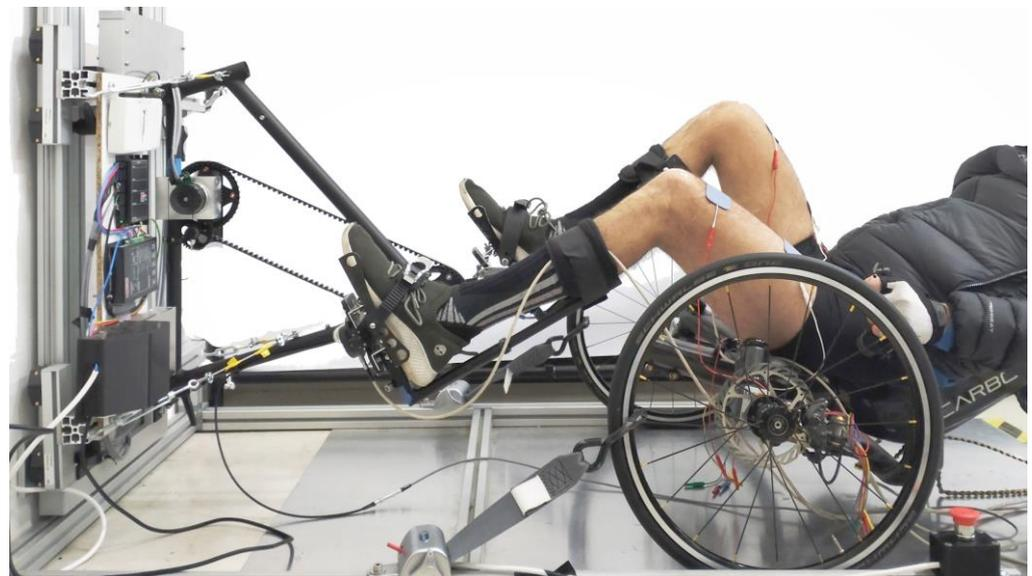
**Figure 3.** Photo of an SCI subject using the platform from the Carbontrike.
