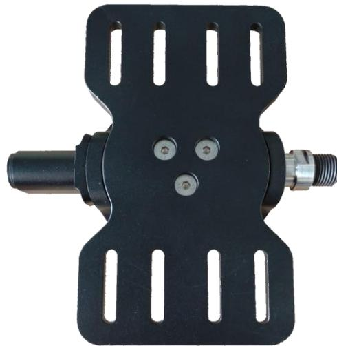
**Figure 2.** A custom connecting plate attached to the force/torque measuring pedal.
