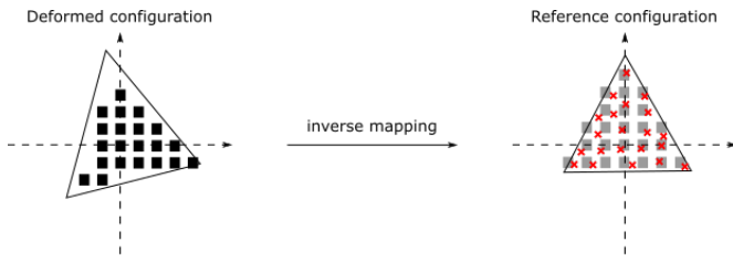
FIGURE 7 Schematic of the deformation procedure of a synthetic image for one triangular element. The black squares depict the pixels positions in the deformed configuration, while the grey squares depict the pixels positions in the reference one. The red crosses denote the pixels from the deformed configuration projected by an inverse mapping in the reference one. The deformed image for the element is obtained by interpolating (bi-cubic spline) the grey levels from the grey squares onto the crosses.
