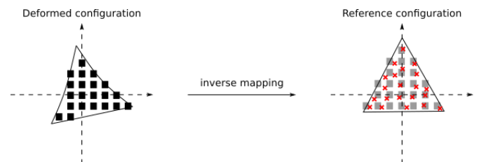
FIGURE 8 Schematic of the deformation procedure of a synthetic image for one triangular element. The black squares depict the pixels positions in the deformed configuration, while the grey squares depict the pixels positions in the reference one. The red crosses denote the pixels from the deformed configuration projected by an inverse mapping in the reference one. The deformed image for the element is obtained by interpolating the grey levels from the grey squares onto the crosses.
