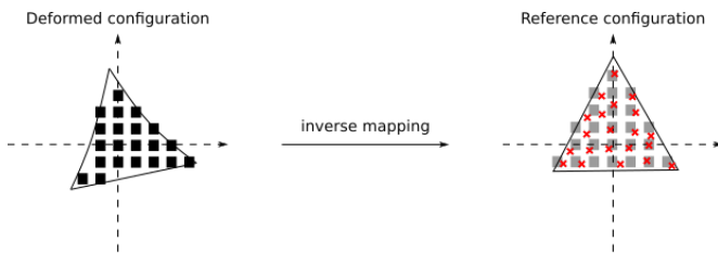
FIGURE 8 Schematic of the deformation procedure of a synthetic image for one triangular element. The black squares depict the pixels positions in the deformed configuration, while the grey squares depict the pixels positions in the reference one. The red crosses denote the pixels from the deformed configuration projected by an inverse mapping in the reference one. The deformed image for the element is obtained by interpolating the grey levels from the grey squares onto the crosses.
