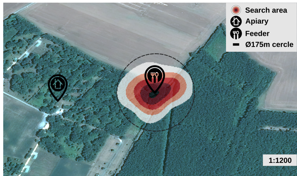
Figure 14. Heat map of the search area deduced from 141 dance vector endpoints decoded by a human observer on 10 min video (21 June 2022) with Pleiade image background (11 June 2022). The position of the feeder is about 230 m east of the GeoDanceHive.
