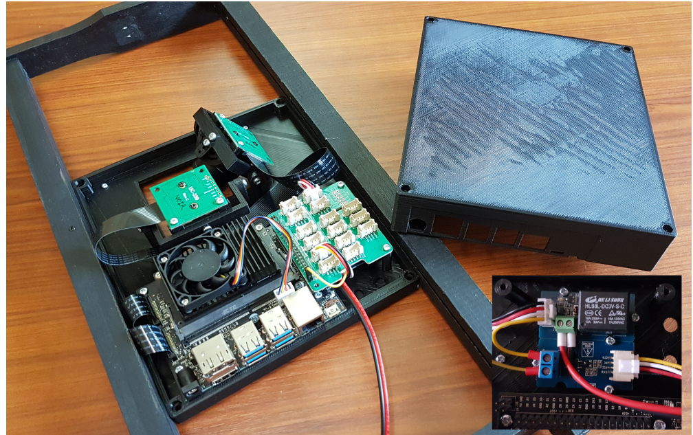
Figure 6. The embedded system with the relays placed under the Grove hat and the two antenna holes in the lower right.
