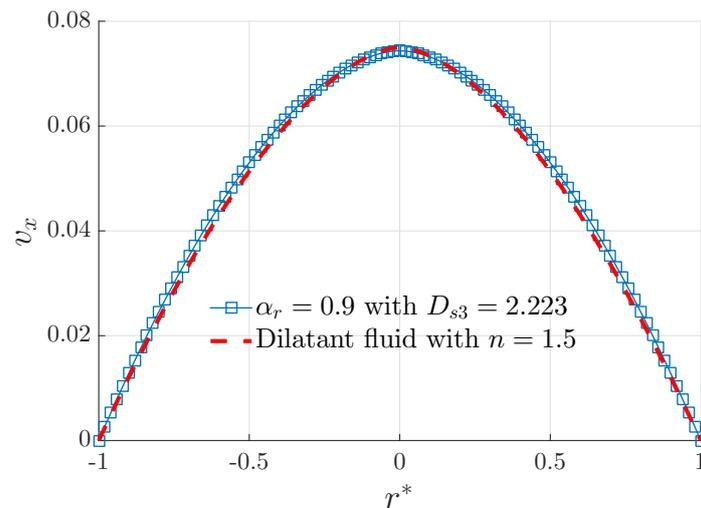
**Figure 8.** Plots of the velocity profile defined by Equation (28) for  $\alpha_r = 0.9$  and  $D_{s3} = 2.223$ , compared with the velocity distribution of a dilatant fluid with index  $n = 1.5$ , with  $r^* = r/r_e$ ,  $d_x = 0.9$ ,  $\Delta p = 25$  Pa,  $\mu = 10^{-3}$  Pa.s, and  $c = 100$  m $^{1-\gamma}$ .
