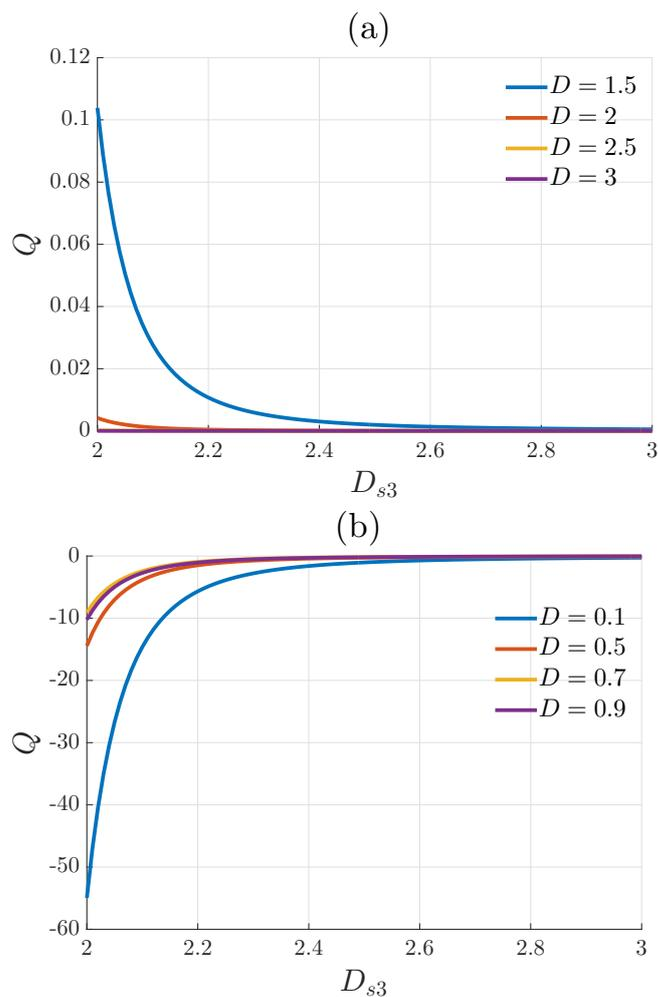
**Figure 9.** Plots of the fractal fluid discharge  $Q$  defined by Equation (35) with respect to the surface fractal dimension  $D_{s3}$  for different values of the mass dimension  $D$ , for (a)  $1 < D \leq 3$ , and (b)  $0 < D < 1$ .  $\Delta p = 25 \text{ Pa}$ ,  $\mu = 10^{-3} \text{ Pa}\cdot\text{s}$ , and  $c = 100 \text{ m}^{1-\gamma}$ .
