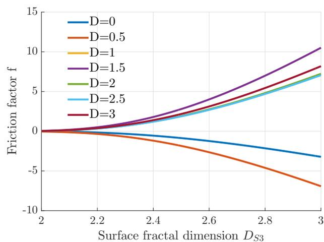
**Figure 10.** Plots of the Darcy friction factor defined by Equation (43) with respect to the surface fractal dimension  $D_{s3}$  for different values of the mass dimension  $D$ , with  $\Delta p = 25 \text{ Pa}$ ,  $\mu = 10^{-3} \text{ Pa}\cdot\text{s}$ , and  $c = 100 \text{ m}^{1-\gamma}$ .
