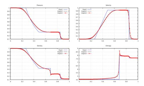
FIGURE 1. Sod shock tube for Euler equations. The CFL are  $CFL_{\rm explicit}=0.4$  and  $CFL_{\rm implicit}=0.4$ .
