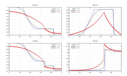
FIGURE 4. Sod shock tube for Euler equations. The CFL are  $CFL_{\rm explicit}=0.4$  and  $CFL_{\rm implicit}=537$  (only one time step).
