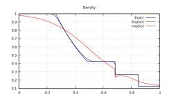
FIGURE 5. Sod shock tube for Euler equations. Mesh of 9000 cells, domain between [-4, 5]. The CFL are  $CFL_{\text{explicit}} = 0.4$  and  $CFL_{\text{implicit}} = 537$ .
