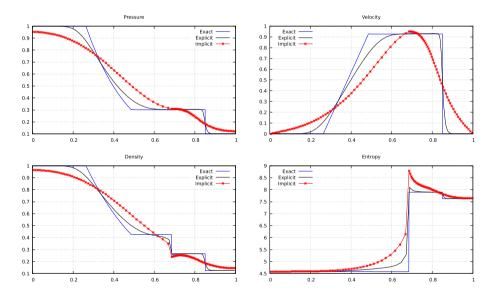
FIGURE 2. Sod shock tube for Euler equations. The CFL are  $CFL_{\rm explicit}=0.4$  and  $CFL_{\rm implicit}=40$ .
