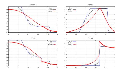
FIGURE 3. Sod shock tube for Euler equations. The CFL are  $CFL_{\rm explicit}=0.4$  and  $CFL_{\rm implicit}=80.$
