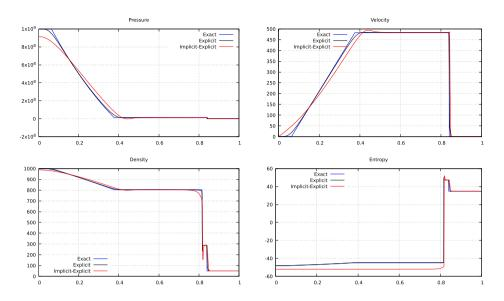
Figure 9. Two-phase shock tube for Euler equations.
